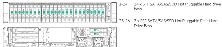
**NOTE:** Drives behind the SAS expander will be labeled continuous, drives behind a controller will be numbered 1-8. **NOTE:** With a SAS Expander and rear drive support the 2SFF rear will be labeled 25 & 26, for 3LFF they will be numbered 25-27.
